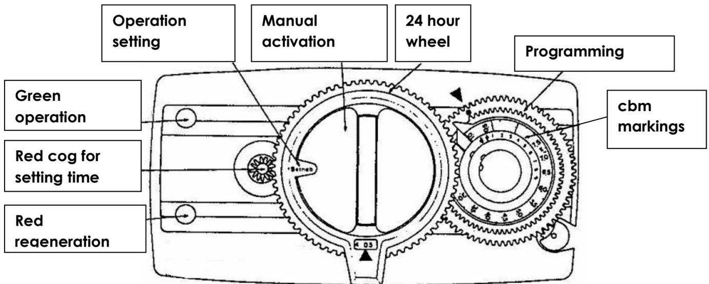
1. Push the red cog for setting the current time. This will release the time setting wheel. Turn this wheel until the little window at the bottom shows the current time at the arrow. Now release the red cog.
